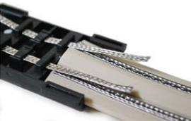
To make a connection, thread the stainless steel braids through the two holes in the Connector and lock the braids in place. The stainless steel braids move current from one track to the next.
