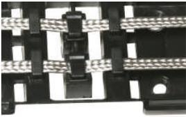
You will need to cut out one side of the centre component. Thread the stainless steel braid through the centre locking snaps. Take the track, slide it into the trough, make sure the stainless steel braid is centred on top of track braid and lock with the snapping caps.
