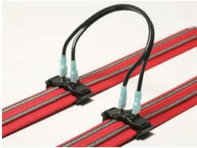
Another part of the E-Quick Connector system is the **E-Quick Tap**. Slide the base under the track and lock it down using the snapping caps. The male connections sticking up will allow you to 'jump' from track to track or to the power charger. A parallel connection between tracks can be accomplished by placing an **E-Quick Tap Jumper Connector** on a track next to the first track and connecting them using lead out wire.
