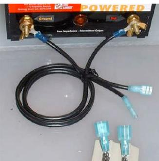
The E-Track and the E-Charger unit are connected using **AVITHOR copper dual lead wire**. This special, highly insulated wire, is available separately. To connect the wire, simply strip the ends of the dual leads and connect the **Ring Connector** to one end and use the appropriate male or female connector to attach the wire to the E-Track.
