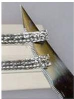
Use a knife to cut the stainless braid free from the track base. Cut back under the stainless steel braid about 15mm.
